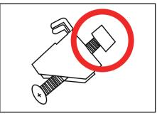
14.Lock the snap nut to the long screw, just lock it flat, do not bulge
