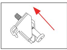
13.Snap screw Installation : First take out the snap screw, use a long screw to twist the screw into the clip inside the direction of the figure.
