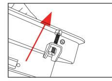
16. Then turn the long screw clockwise onto the snap plate to fix the machine. Generally, the two snap screws on the left and right sides
